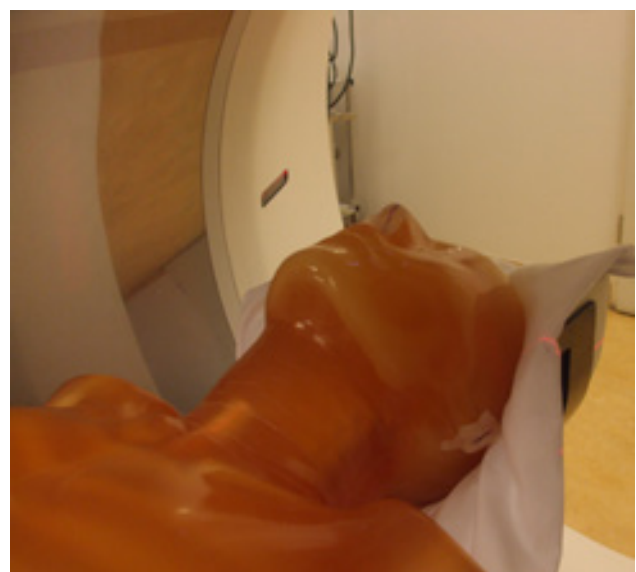
(Figure 3) CT Torso Phantom CTU-41 Positioned in the CT-Scan.
