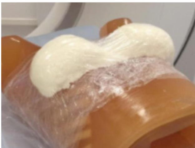
Figure 1: Lungmann with an attached custom-designed breast phantom.
