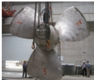
Large-diameter bulb water turbine runner for China
