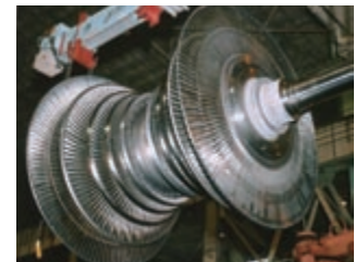
High-performance steam turbine rotor for the Geysers Power Plant, U.S.A.
