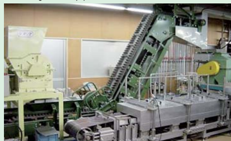
Separation and classification equipment manufactured in-house (It sorts waste into metal, glass and mercury.)
